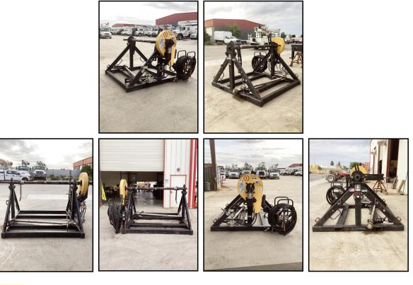
Reel OD Capacity: 102 Inches **Reel Width Capacity: 70 Inches**
