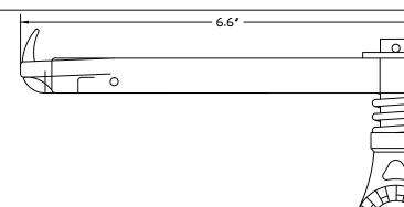
USED TO PARTIALLY WITHDRAW A BALL-SOCKET COTTER KEY SO THAT THE INSULATOR CAN BE REMOVED FROM ANOTHER INSULATOR HANGER. IS PREFERRED FOR PRYING STANDARD KEYS DEEPLY SET ON LONG INSULATORS STRINGS,
