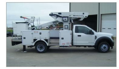
EQUIPMENT SPECIFICATIONS: VERSALIFT VST-40-1 WITH A WORKING HEIGHT OF 45' AND HORIZONTAL REACH OF 30' SIX GPM OPEN CENTER HYD SYSTEM W/ A 3000 PSI OPERATING PRESSURE SIDE MOUNTED TELESCOPIC UPPER BOOM FIBERGLASS INNER BOOM FIBERGLASS LOWER BOOM BOOM INSERT NON-LUBE BEARINGS OUTRIGGER BOOM INTERLOCK SYSTEM 17 GAL RESERVOIR INDIVIDUAL FULL PRESSURE CONTROLS AT THE TURRET ACTUATE WITH A SELECTOR VALVE TO OVERRIDE UPPER CONTROLS 12V DC BACKUP PUMP AUTO THROTTLE CONTROL SAFETY HARNESS AND LANYARD
