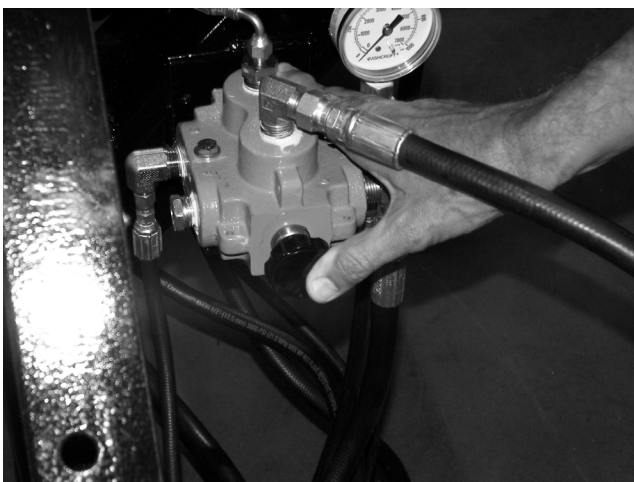
Figure 4. Push in Selector Valve Handle
