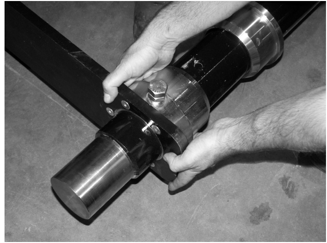
Figure 12. Remove Lifting Bracket
