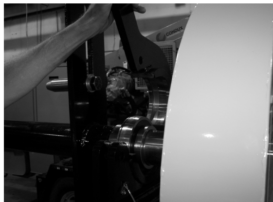
Figure 10. Open Bearing Keeper to Fully Open Position
