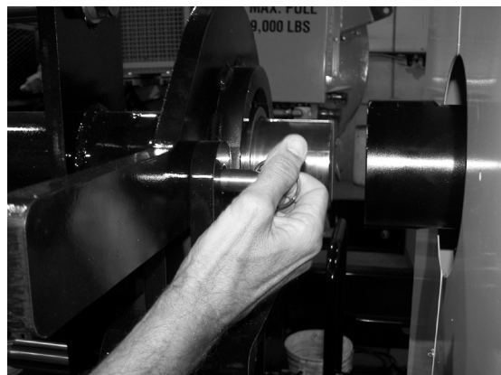
Figure 9. Remove Retainer Pin from Bearing Keeper
