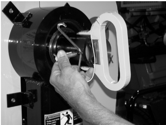
Figure 7. Remove Keeper Pin from Drive Pin
