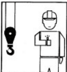
EXTEND BOOM - (Telescopic Booms) One Hand Signal. One fist in front of chest with thumb tapping chest.
