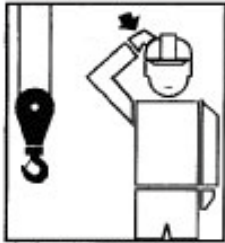
USE MAIN HOIST - Tap fist on head; then use regular signals.
