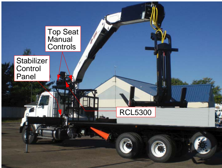
24562/28562 Crane Controls Locations (shown with top seat)
