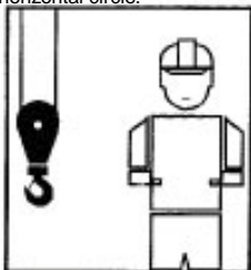
RETRACT BOOM - (Telescopic Booms) Both fists in front of body with thumbs pointing inward.
