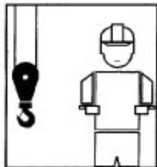
EXTEND BOOM - (Telescopic Booms) Both fists in front of body with thumb pointing outward.
