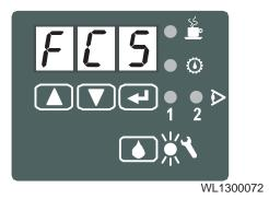
Figure 63 Fault notification on device display
