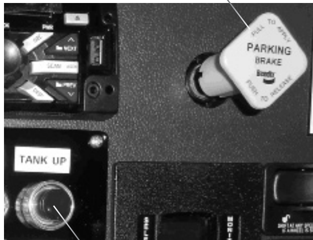
“Tank Up” Light and Alarm
