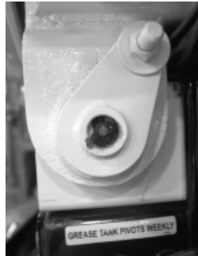
19 - DEBRIS TANK PIVOT PINS
