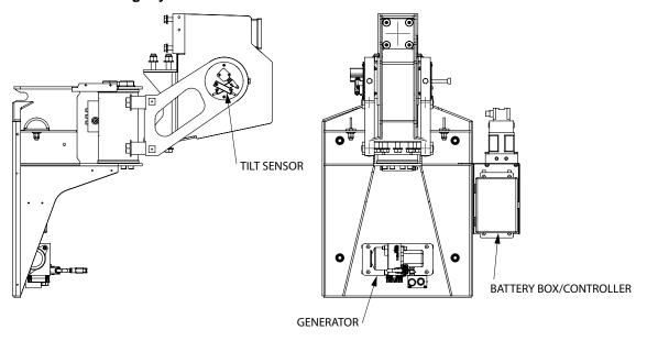
If the platform is more than 15 degrees out of level the level control system will turn off and not level until it is manually leveled to less then 15 degrees from level position.
