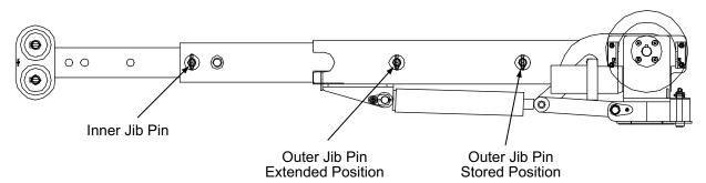
Both the 1st inner and 2nd outer jib extensions are manually operated. To extend the inner jib section:
