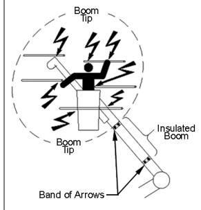
The insulating boom section only prevents current from passing from the band of arrows at the boom tip to the lower band of arrows. All components above and below that area must be considered conductive.
