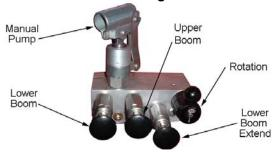
NOTE: The handle for the manual hydraulic pump is located above and to the left of pump, fixed to the adjacent cover. This picture illustrates the Manual Let Down System without the covers in place.
