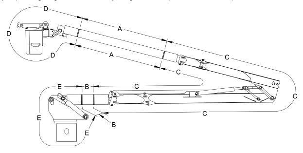
**Area A.** Upper Boom Insulation, provides an insulating area between area D and earth ground when in properly maintained condition.
