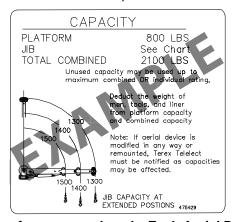
NOTE: Load charts shown are for an example only. Each Aerial Device has its custom made load chart which may have different capacities than shown here.
