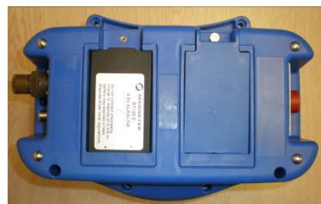
Figure 2: Installation of battery.
