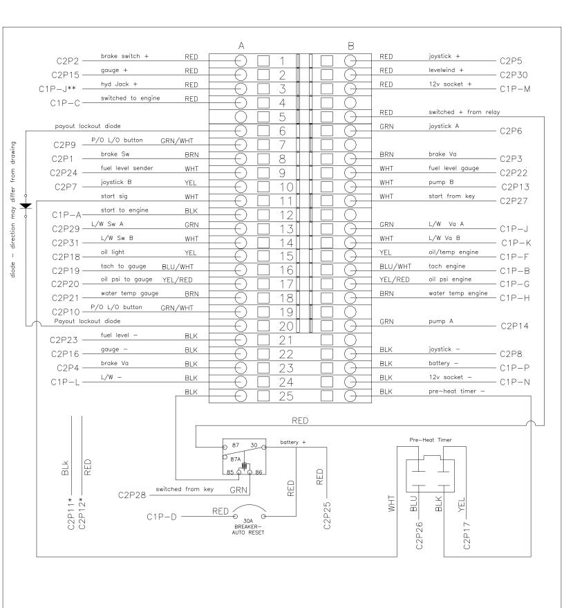
\* 2nd coil from M90 pump \*\* Pin is OPTINAL power wire for HYDRAULIC OUTRIGGERS \*\*\* Pins are for OPTIONAL TOOL CIRCUIT
