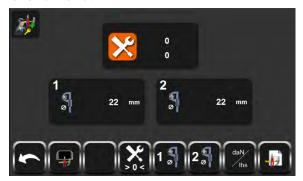
This screen indicator represents the maintenance due notification, showing the client when the next maintenance is due. If the maintenance is due, the pictogram is displayed in orange. Otherwise, the pictogram is displayed in grey.
