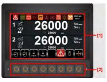
on and the system loads, the first screen the operator sees (after the S+R™ logo screen) is the **MAIN MENU screen**. This screen allows the operator to access the functions of the system, while also allowing access to settings and diagnostics.
