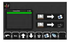
This screen allows the operator to see information related to the storage and transfer of recorded system data logs.
