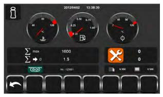
At the top of this 2012/04/02 13:38:30 display resides the date and time bar. This bar provides the current date and time-based on what is set in the system.
