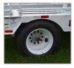
monitored, as heavy trailer weight on low tires can create permanent buckling of the tire sidewall resulting in the need for tire replacement.
