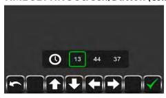
To change the time in the system, use the right and left arrow buttons to move the green selection box between Hour, Minute, and Second intervals. Once an interval is selected, use the Up and Down arrow keys to adjust the number up or down.
