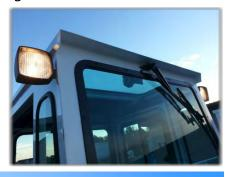
**NOTE:** The master power key switch must be turned to the on position to activate the exterior work lights.
