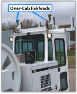
✓ Once the conductor end is through the fairleads and in reach of the reeving rope, tie the conductor end(s) to the reeving rope end(s).
