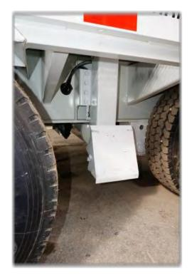
**CAUTION:** Ensure that all jacks are fully raised and clear of the ground before attempting to tow trailer.
