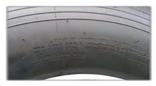
**CAUTION:** Replacement tires must meet the same specifications as the originals. Tires for Sherman+Reilly™ machines meet specific duty requirements, as well as weight and roadway/speed ratings. Mismatched tires and rims may come apart with explosive force causing personal injury. Mismatched and underrated tires can also blow out causing vehicle and roadway accidents that can create serious injury or death for those involved.
