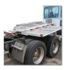
✓ With operators cab closed and locked, position hand rails so that they overlap the doors. Tighten handrails in place to help hold doors closed during transit.
