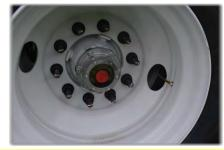
**CAUTION:** Wheel nuts or bolts must be tightened and maintained at the proper torque levels to prevent loose wheels, broken studs, and potential dangerous separation of the wheel from the axel, which can cause accidents, personal injuries, and death.
