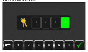
There are two menus within the ADDITIONAL SETTINGS Screen: **Client Menu** and **Service Menu**. Each menu has an independent password; therefore, to access each menu the user must enter the specific password for that menu-Client or Service.
