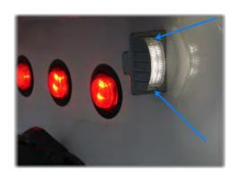
✓ <u>Unscrew</u>: Some lighting may require the use of a screw driver to unscrew the light from its housing.
