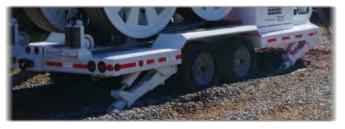
**CAUTION:** Ensure that all jacks are fully raised and clear of the ground before attempting to tow trailer.
