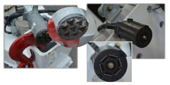
✓ Also, check lighting junction box for damage. Open and inspect wires for loose or corroded connections.
