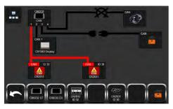
The selection buttons at the bottom of this screen represent communication components, and they may vary across different models and versions of the machine. Press the individual buttons to open the I/O pages of each different communication component.
