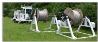
**NOTE:** The reel stand hydraulic controls should be in the disengaged or Off/Closed position when not in use.
