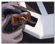
✓ <u>Pop Tabs</u>: Some lighting may require the use of a screw driver to unsnap the light from its retaining tabs.
