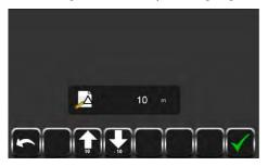
To increase the frequency of recording segments, reduce the length by pressing the Down arrow button. To decrease the frequency of recording segments, increase the length by pressing the Up arrow button.
