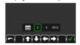
To change the date in the system, use the right and left arrow buttons to move the green selection box between Month, Day, and Year intervals. Once an interval is selected, use the Up and Down arrow keys to adjust the setting up or down.
