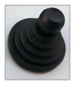
(away from the operator) on the joystick. The farther away from the center point the joystick is moved in either direction, the faster the bullwheels will turn, thereby increasing line speed. To slow the line speed from either payout or pulling directions, move the joystick closer to the center point. Once the joystick reaches the center point, the bullwheel motion and line speed will stop, and the hydraulic brake will set.
