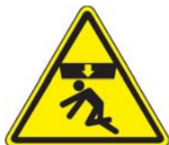
Crushing of body hazard
