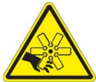
Cutting and/or crushing hazard
