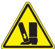
Crushing of Foot Hazard
