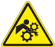
Pinch point and/or entanglement hazard
