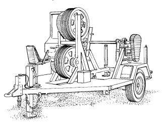
2. The unit should be set up as level as possible, centered on the lead block and parallel to the line being pulled. Chock or block the trailer tires on both sides and disconnect from the tow vehicle. Level the unit using all three jacks.
