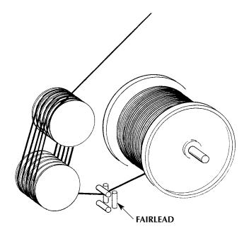
3. Standing at the front of the machine, facing toward the rear of the machine, the conductor should lead through the fairlead into the bottom of the left hand groove of the lower bullwheel. The conductor should be reeved in each bullwheel groove and leave the top right hand groove of the upper bullwheel going to the pole over the conductor reel and rear of the machine.
