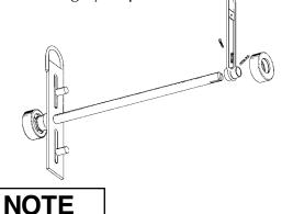
The conductor reel should be placed so that the conductor will feed off the bottom of the reel, through the fairlead window, to the front of the machine.
