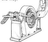
3. Use a spreader bar on the chains to the lifting device to lift the reel and drive bar assembly up out of the pillow block housing.
