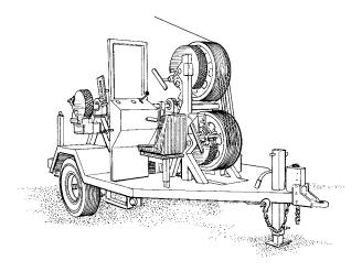
The machine is equipped with reel locking pins. They should be engaged when transporting the reel or when leaving the conductor under tension for long periods of time.
