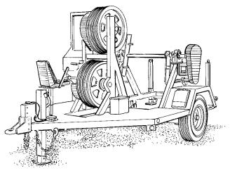
The drive motor is operated with a three-position control lever which returns to neutral when released.
