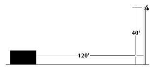
**Example:** If the first structure/pole is 40 feet high, it is recommended the puller be approximately 120 feet from the base whenever possible.
