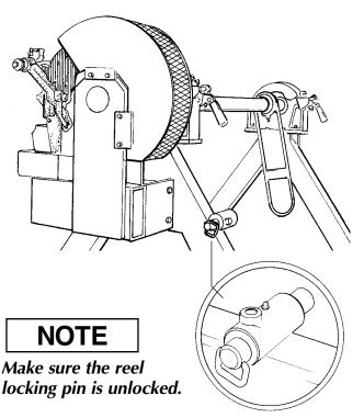
2. Remove the locking pins and unlatch the pillow block housing on both sides. Rotate the top of the housing to the full open position and make sure the latch is folded back out of the way.
