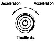
[A] Hand throttles switch (mounted at the top of the swing lever)
