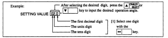
In the above example, "0" is inputted to the first decimal digit, "2" to the units digit and "0" to the tens digit and so the boom lower limit gentle operation angle is set to 2°. If the gentle operation is not necessary, set the angle (0.00). Normally, the standard is approximately 2°.
