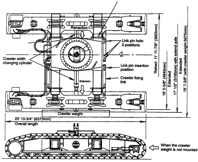
Change the crawler width by extending or retracting the crawler width changing cylinder. Retract the crawler width fully, and the overall crawler width is 11' 11-7/8" (3655mm). Extend the crawler width to the middle position, and the overall crawler width is 16' 2-5/8" (4945mm). Set the crawler width to the maximum extension position, and the overall crawler width is 17'-1/2" (5195mm). When you want to set the crawler width to 17'-1/2" (5195mm), the extension axle must be attached to the axle.
