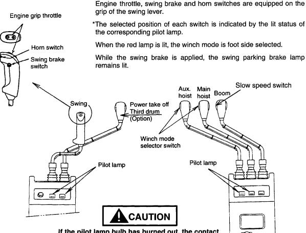
If the pilot lamp bulb has burned out, the contact is not good, the wire is out of position or disconnected, the indicator is not working and an operation error may be caused. Before starting the operation, perform a lamp test by turning the ignition switch to the "ON" position.
