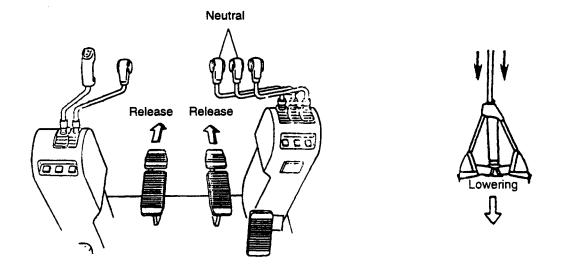
Release both the closing brake and the holding brake, and gently lower the bucket onto the substance to be dug.
