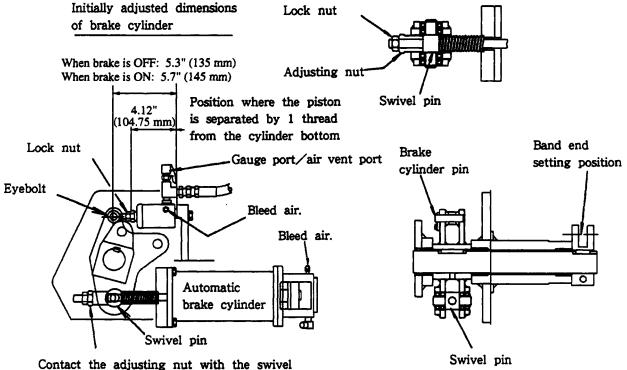
contact the adjusting nut with the swivel pin tightly when the rod is extended to the maximum by supplying the pressurized oil to the cylinder.
