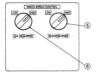
Set the switch to "LOW", and the load hoist drum rotation is decelerated. Set it to "HIGH", and the load hoist drum rotation is accelerated. Don't change the hoisting speed during hoisting or lowering. Stop the load and apply the brake securely before changing the speed.
