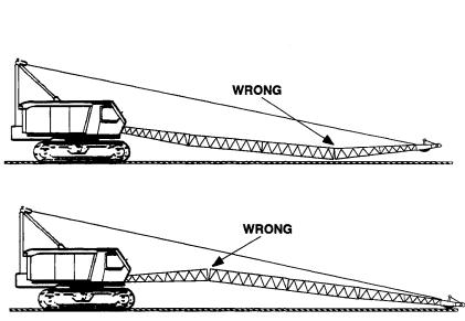
B. Boom Disassembly with Service Crane
