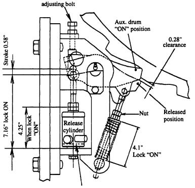
When the cylinder dimension is 4.25", keep a clearance of 0.2" between the cylinder bottom and piston.
