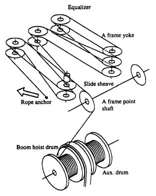
Spool off the wire rope while turning the reel to prevent twisting. Wind the rope around the sheave without crossing it. When winding the wire rope around the boom hoist drum, give prestress to the rope and wind it correctly for the first layer on the drum.
