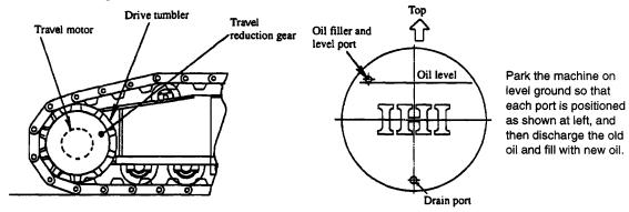
Oil can be discharged easily when it is still hot, shortly after operation.
