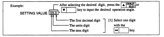
In the above example, "0" is inputted to the first decimal digit, "3" to the units digit and "0" to the tens digit and so the boom lower limit gentle operation angle is set to 3°. If the gentle operation is not necessary, set the angle (0.00). Normally, the standard is approximately 2°.
