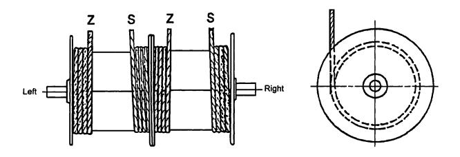
The wire rope tends to turn in the untwisting direction when it is tensed. When winding the first layer of rope evenly by pulling strongly as shown above, it serves as a basis for subsequent correct winding. If the rope is wound roughly on the first layer, it is overlaid one-sidedly or bitten between adjacent ropes, causing excessive wear or crushing. As a result, the rope will reach the end of its service life earlier.
