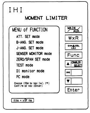
When pressing the Enter key, the displayed values are stored as the new set data and the function selection menu is automatically displayed.
