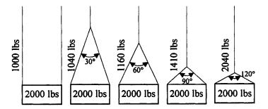
If an angle is formed between ropes as shown above, the safety factor must be multiplied with the determined coefficient. At a rope hooking angle of 60° a coefficient of 1.16 must be used. Also, the safety factor of hoisting chain is specified to 5 or more. Periodic checking and the service limit are also determined for slinging devices. Carry out their periodic check. Never use damaged sling wire rope.
