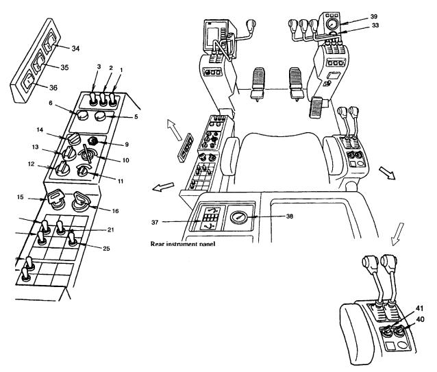
Set the switch of the winch to be used to "ACTIVE". If not, the overhoist prevention device will not work. Set the switch of the unused winch to "RELEASE". The switches are positioned above the control panel behind the operator's cab.
