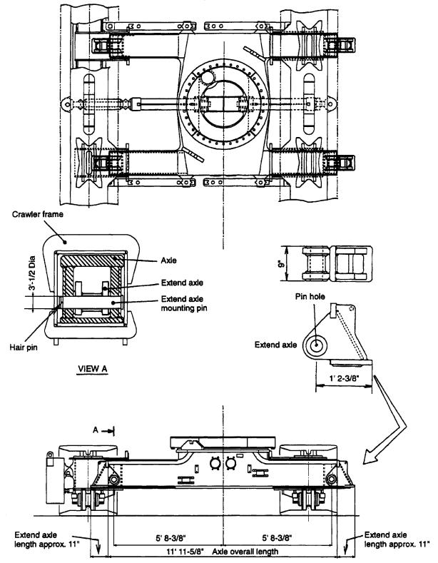
When the extension axle is mounted, one side of the axle is lengthened by approx. 11"
