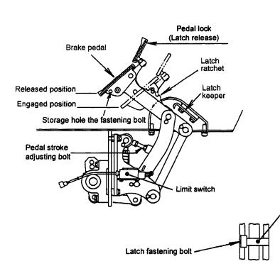
Operation of drum lock (main drum lock structure)
