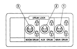
These are the drum lock switches for main hoist, auxiliary hoist and boom hoist. Set the switch to the key release position, and the drum is unlocked. Hoist the drum a little if it is difficult to unlock the drum. Force is removed from the pawl and the drum is unlocked.
