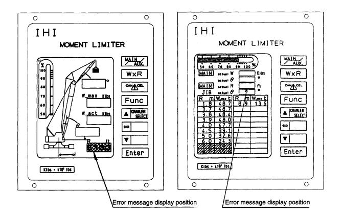
In both of the above illustrations, the error message is displayed as "E100" on the working radius column. "E100" blinks and an alarm is heard. Refer to "Error Code Table" for the causes and remedial measures of the errors.
