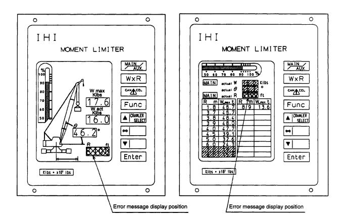
In both of the above illustrations, the error message is displayed as "E100" in the working radius column. "E100" blinks and an alarm is heard. Refer to "Error Code Table" for the causes and remedial measures of the errors.
