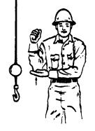
USE WHIPLINE (Auxiliary Hoist). Tap elbow with one hand, then use regular signals.
