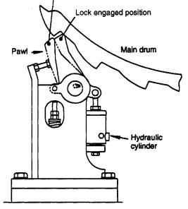
For releasing the brake, separate the latch ratchet from the latch keeper by depressing the latch release and allow the pedal to rise. Usually, the pedal is moved up and down while depressing the latch release.
