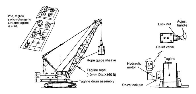
If the tensile force is excessive, the bucket is pulled toward the operator, and it is swung outside if the force is inadequate. It will be an overload, if a work radius increased, so be careful. Adjust the tensile force so as to match the working state.
