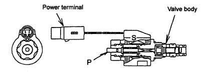
Electromagnetic proportional relief valve controlling hydraulic pump
