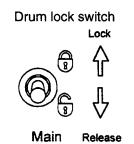
Before hoisting or lowering, the drum lock must be disengaged. When tilting the release position of the lock switch on the left control panel, the relevant drum is unlocked. Upon turning the switch to the release position, oil pressure is sent to the hydraulic cylinder so the pawl is disengaged from the drum.
