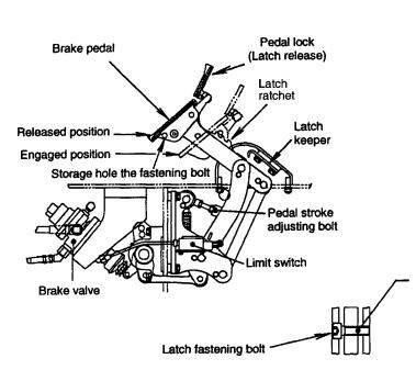
Operation of brake pedal (auxiliary drum structure)
