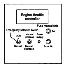
If a problem occurs in the control system, turn the auto/manual selector switch of controller to the "Manual" position. Then, the engine speed can be increased or decreased by the manual increase/decrease switch.
