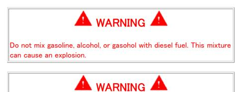
Under no circumstances must gasoline or alcohol be used to dilute diesel fuel. This practice creates an extreme fire hazard and under certain circumstances an explosive hazard. Gasoline dilution is not an effective way to lower cloud point (20 volume-percent gasoline only lowers cloud point 4° C [7° F] and it lowers the fuel viscosity, cetane number, and flash-point). Alcohol dilution will increase the cloud point.
