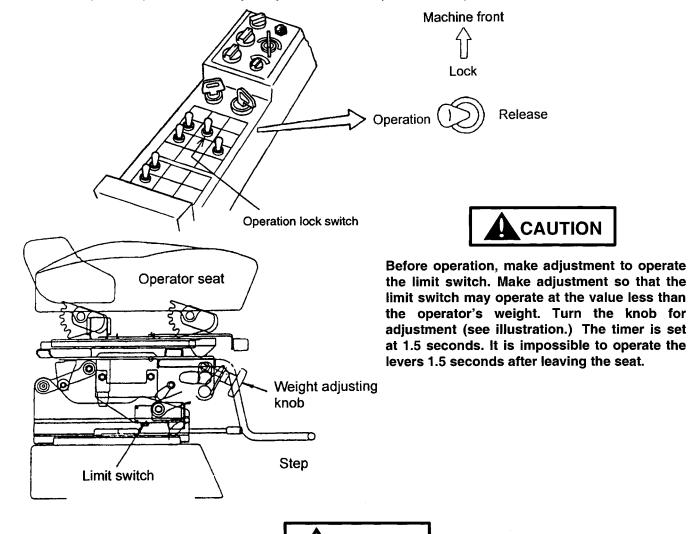
1. This device does not function when the operation lock switch of the left operation console is turned to the released position. For safety this switch must be set to the operation position.
