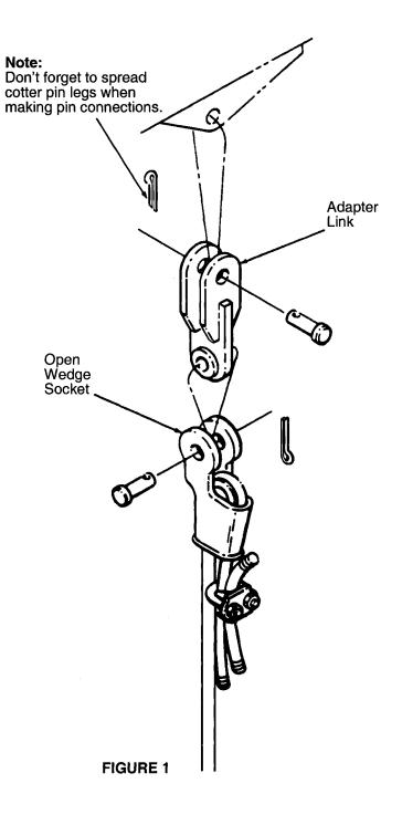
REFER TO THE PROCEDURE FOR "SECURING THE DEAD END OF A ROPE WHEN USING A WEDGE SOCKET" IN THIS MANUAL (PAGES 2-43 & 2-44).
