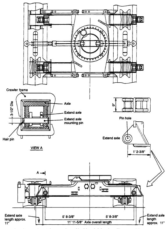
When the extension axle is mounted, one side of the axle is lengthened by approx. 11"
