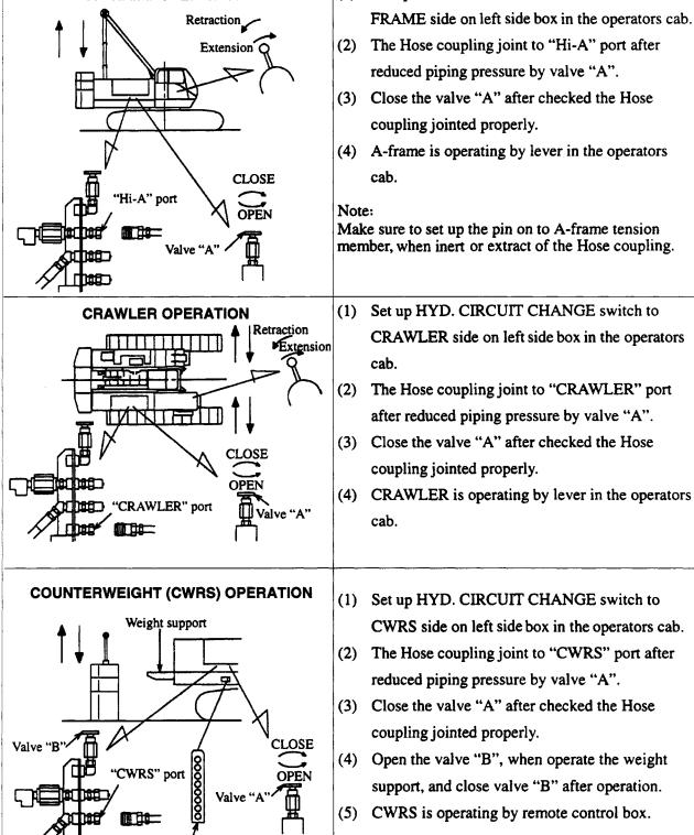
Do not change the joint of piping and electric wiring when the engine is running. Printed in U.S.A. Page 2-26 1/01
