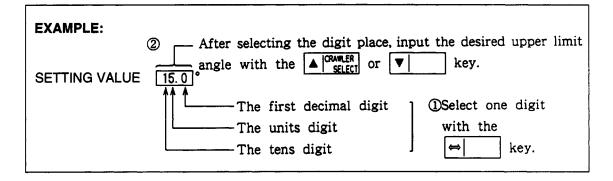
In the above example, "0" is inputted to the first decimal digit, "5" to the units digit and "1" to the tens digit, and so the jib optional offset upper limit angle is set to 15.0°. Set this angle to 10.0° if not necessary.
