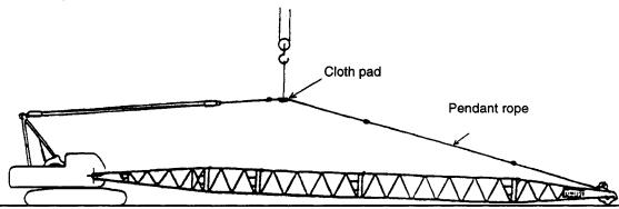
Use a pad for the lifted section of the pendant rope so as not to make an extreme bend in the rope. Gradually lift the next pendant rope in addition to the first one. For the tower crane, carry out the above procedure if necessary.
