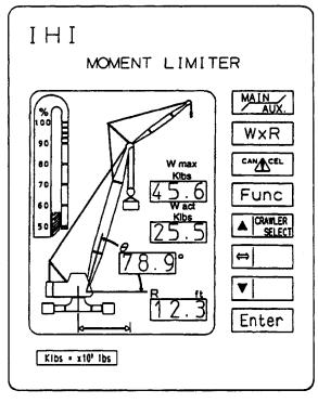
OPERATION TRANSPORT ERECTION Moment limiter mode switch (Refer to Page 1-9)
