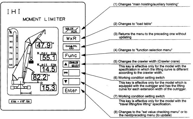
(1) Main/auxiliary selector key switch MAIN Press the main/auxiliary selector key switch MAIN , the main hoisting work menu is changed to the auxiliary hoisting work menu. Press the MAIN key again, and the menu is changed to the main hoisting work menu. Select a proper menu according to the actual crane configuration. It is not permitted to lift loads with the main hook and the jib hook at the same time.
