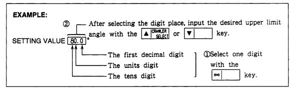
In the above example, "0" is inputted to the first decimal digit, "0" to the units digit and "8" to the tens digit, and so the boom optional upper limit angle is set to 80.0°. Maximum upper limit angle is 90.0°.
