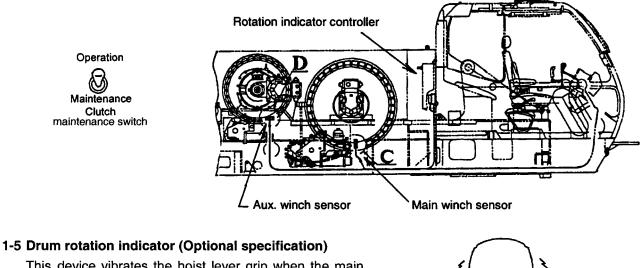
This device vibrates the hoist lever grip when the main or auxiliary winch drum rotates and so indicates the drum rotation for the operator. The vibration stops when the drum rotation reaches the specified or higher value.
