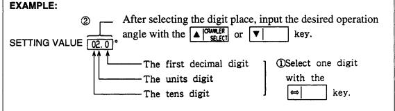
In the above example, "0" is inputted to the first decimal digit, "2" to the units digit and "0" to the tens digit, and so the boom lower limit slow-down angle is set to 2.0°. If the slow-down operation is not necessary, set the angle (0.00). Standard minimum slow-down angle is approximately 2.0°.
