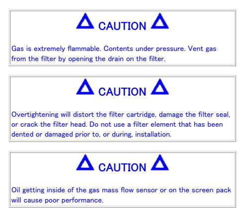
Fuel filters are required equipment on all Cummins® natural gas engines. They are designed to remove oil and harmful particles from the fuel before they damage the fuel system or other engine components. These filters are a coalescent type filter that will capture oil contaminants and moisture typically found in natural gas.
