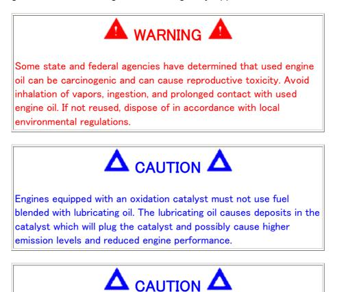
Do not blend more than 5 percent used lubricating oil with the fuel. Do not blend other used oils with fuel, such as transmission fluid, gear case oil, and so forth.
