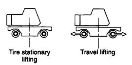
This key switch works when tires are used for the travelling unit. Press the key once, and the displayed picture is changed to "travel lifting". Press the key again, and the displayed picture is changed to "tire stationary lifting".
