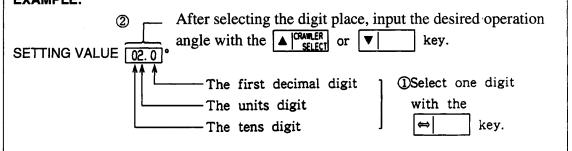
In the above example, "0" is inputted to the first decimal digit, "2" to the units digit and "0" to the tens digit, and so the boom lower limit slow-down angle is set to 2.0°. If the slow-down operation is not necessary, set the angle (0.00). Standard minimum slow-down angle is approximately 2.0°.
