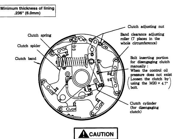
Before adjusting or repairing the brake or clutch, the hook block and suspension load must be lowered to the ground. Lower the boom if necessary for safety.
