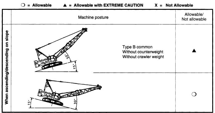
Allowableness is shown for the machine with counterweight and without counterweight.
