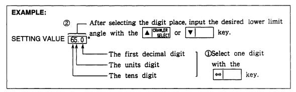
In the above example, "0" is inputted to the first decimal digit, "5" to the units digit and "6" to the tens digit, and so the boom optional lower limit angle is set to 65.0°. Minimum lower limit angle is 60.0°.
