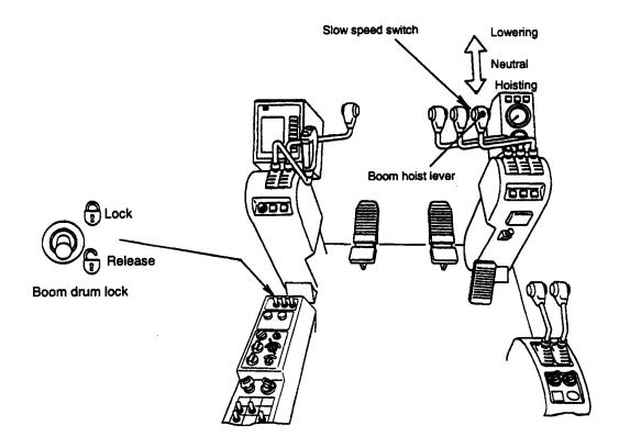
While the boom is hoisted or lowered, the disc brake built into the hydraulic motor is automatically released and the brake is automatically applied to stop and hold the boom when the lever is set at neutral.
