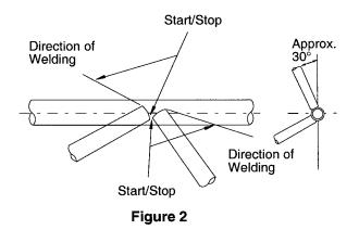
**Note:** Weld 1st side Toe to Heel and 2nd side Heel to Toe.
