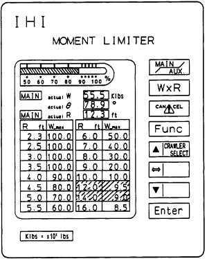
[1] Press the WxR switch once on the standard menu, and the load table is displayed. On the load table display, press the WxR or CANACEL key once and the standard menu appears.
