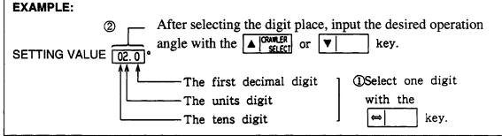
In the above example, "0" is inputted to the first decimal digit, "2" to the units digit and "0" to the tens digit, and so the upper limit slow-down angle is set to 2.0°. If the slow-down operation is not necessary, set the angle (0.00). Normally, the standard minimum slow-down angle is 2.0°.
