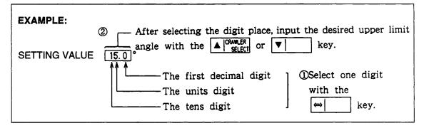
In the above example, "0" is inputted to the first decimal digit, "5" to the units digit and "1" to the tens digit, and so the jib optional offset limit angle is set to 15.0°. Set this angle to 10.0° if not necessary.
