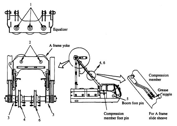
The yoke shaft and connection link should be greased through the above grease pipe.
