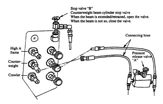
Set the hydraulic circuit selector switch (29) to "CWRS CYLINDER" beforehand. When the switch is in this position, change the hose connection as the above and mount/remove the counterweight. When operating the high A-frame and changing the crawler width, set this selector switch to "A-FRAME".
