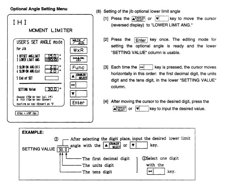
In the above example, "0" is inputted to the first decimal digit, "0" to the units digit and "3" to the tens digit, and so the jib optional lower limit angle is set to 30.0°. Set this angle to 15.0° or lower if not necessary.
