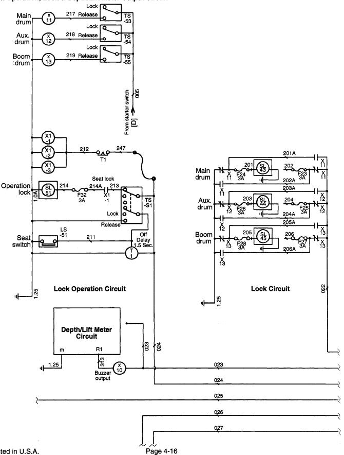
Lock Operation, Lock & Depth/Lift Meter Output Circuit
