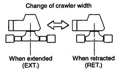
On the machine without the crawler width change specification, set the crawler width to the extended position. If the crawler width is retracted, "E114" is displayed and the alarm sounds. This key switch does not work on the wheel type. (6) The key switch to change the outrigger width ↔
