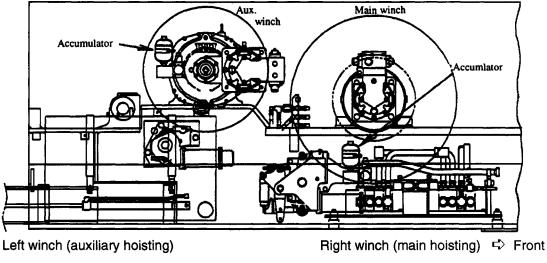
Line filter and accumulator mounting positions
