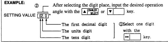
In the above example, "0" is inputted to the first decimal digit, "2" to the units digit and "0" to the tens digit, and so the upper limit slow-down angle is set to 2.0°. If the slow-down operation is not necessary, set the angle (0.00). Standard minimum slow-down angle is 2.0°.
