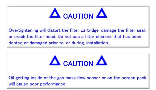
Fuel filters are required equipment on all Cummins® natural gas engines. They are designed to remove oil and harmful particles from the fuel before they damage the fuel system or other engine components.
