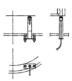
The clearance between drum and a sensor is adjusted to 0.102"
