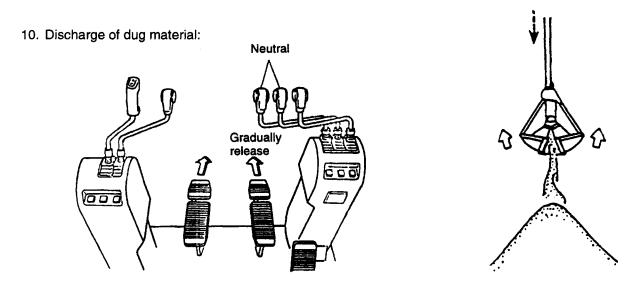
When the bucket comes to the determined position, return both levers to neutral with the closing and support brake pedals depressed. Discharge the dug material by gradually loosening the closing brake. Pay attention not to loosen the brake excessively, otherwise the wire rope is loosened unnecessarily, causing irregular winding.
