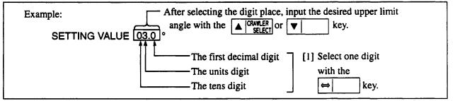
In the above example, "0" is inputted to the first decimal digit, "3" to the units digit and "0" to the tens digit and so the upper limit gentle operation angle is set to 3°. If the gentle operation is not necessary, set the angle (0.00). Normally, the standard is approximately 2°.
