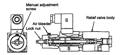
Pressure is set by turning the adjustment screw with the lock nut loosened. Normally, return the screw completely and be sure to tighten the lock nut.
