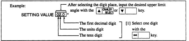
In the above example, "0" is inputted to the first decimal digit, "2" to the units digit and "0" to the tens digit and so the upper limit gentle operation angle is set to 2°. If the gentle operation is not necessary, set the angle (0.00). Normally, the standard is approximately 2°.
