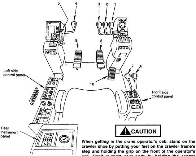
crawler shoe by putting your feet on the crawler frame's step and holding the grip on the front of the operator's cab. Don't support your body by holding the control levers when getting in or out of the operator's cab. If the operation lock switch is at the release side, the crane function will move by moving the lever.
