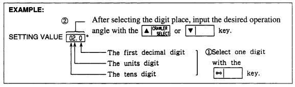
In the above example, "0" is inputted to the first decimal digit, "2" to the units digit and "0" to the tens digit, and so the upper limit slow-down angle is set to 2.0°. If the slow-down operation is not necessary, set the angle (0.00). Standard minimum slow-down angle is 2.0°.
