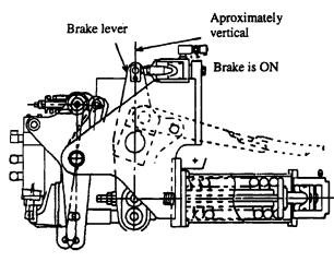
4. Adjustment of the brake band tension
