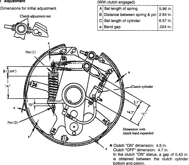
Usually, the clutch is adjusted for wear of the lining. If the clutch has been disassembled for repair, etc., the above dimensions for initial adjustment should be obtained. Follow the procedure given below.
