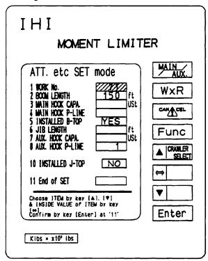
(3) Set the working condition on the setting menu. Press the ▲ CRAWLER or ▼ key to move the cursor to "WORK No." The item with the cell is
