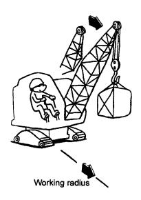
If the load is lowered onto the ground in working at the upper limit boom angle (80°), the automatic boom stopper may be activated. Pay attention!
