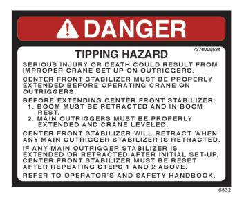
Carefully follow the procedures in this Operator Manual when extending or retracting the outriggers. Death or serious injury could result from improper crane setup on outriggers.
