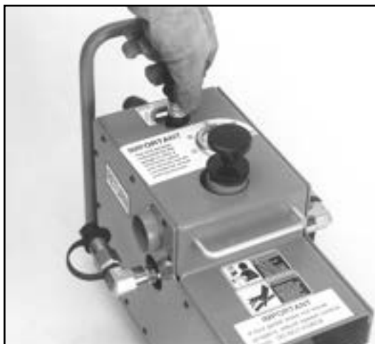
Figure 22. Pressure Relief Valve
