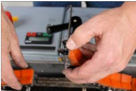
11. Pass the pre-lubricated new chain around the drive sprocket. Feed the chain along the unit and reconnect the chain-connecting link. Remember to install the 2 center connecting link plates.
