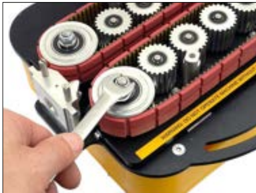
loosen and remove the tension nuts
