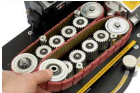
remove the idler pulleys and the belts
