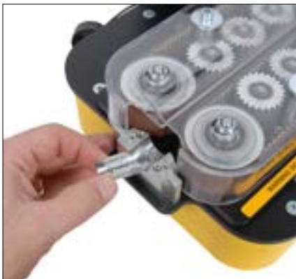
Remove and replace the guide
