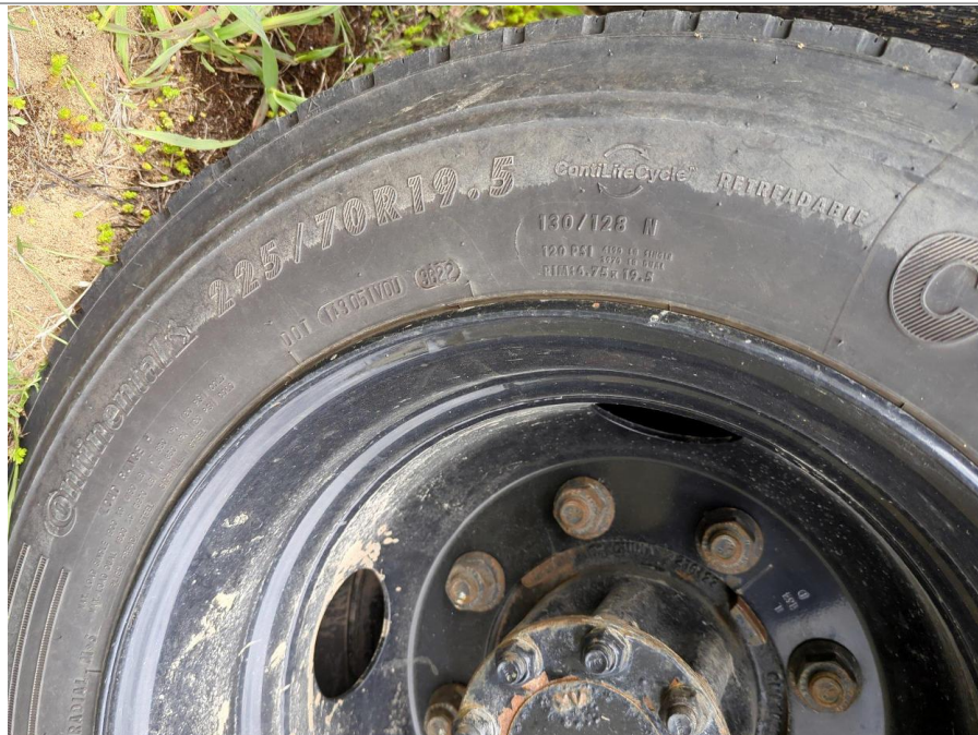
First Right Outer Drive Tire Size
