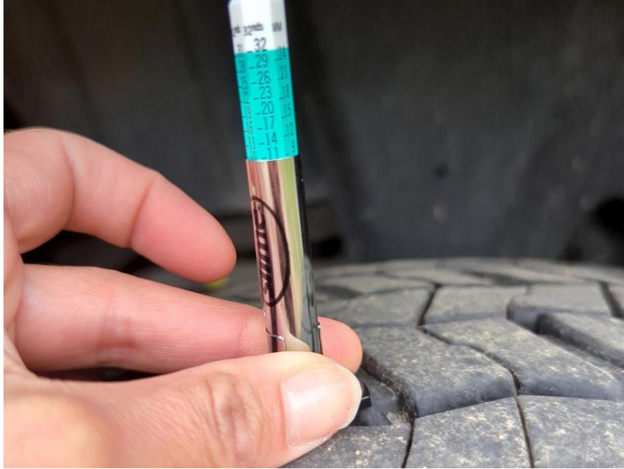
First Left Steer Tire Tread Depth Measurement
