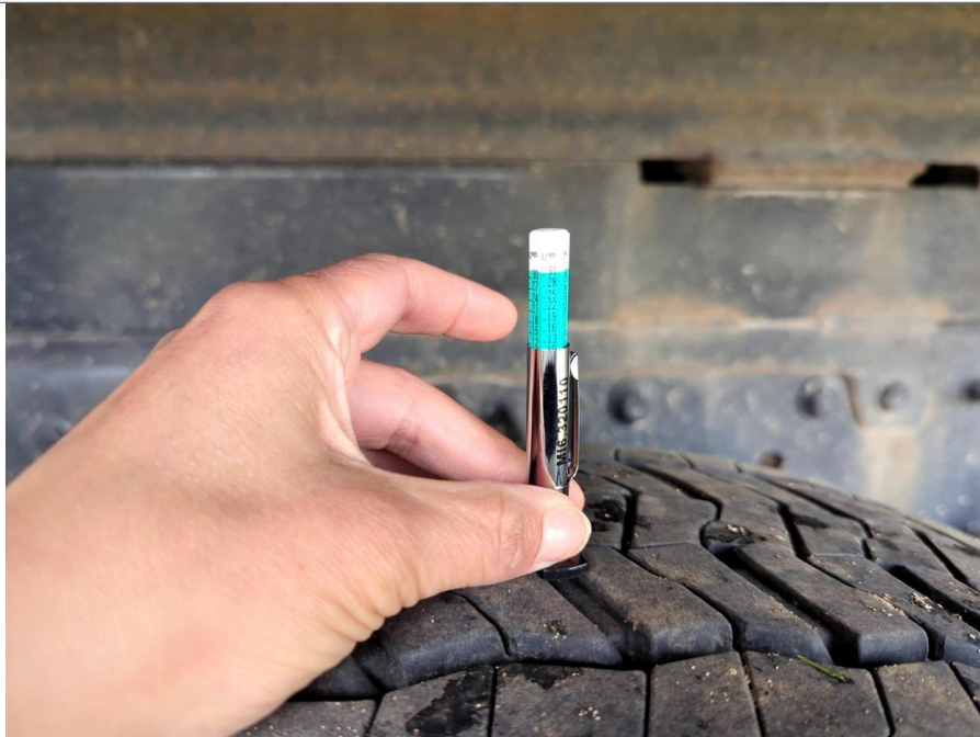
First Right Inner Drive Tire Tread Depth Measurement
