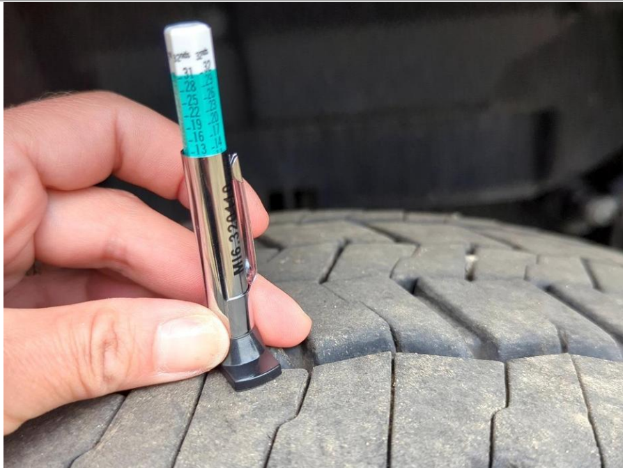
First Right Steer Tire Tread Depth Measurement
