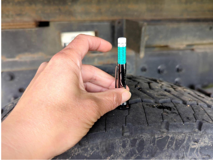
First Left Inner Drive Tire Tread Depth Measurement
